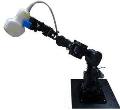
Fig. 5. Developed robotic arm with 3D position memory function.
